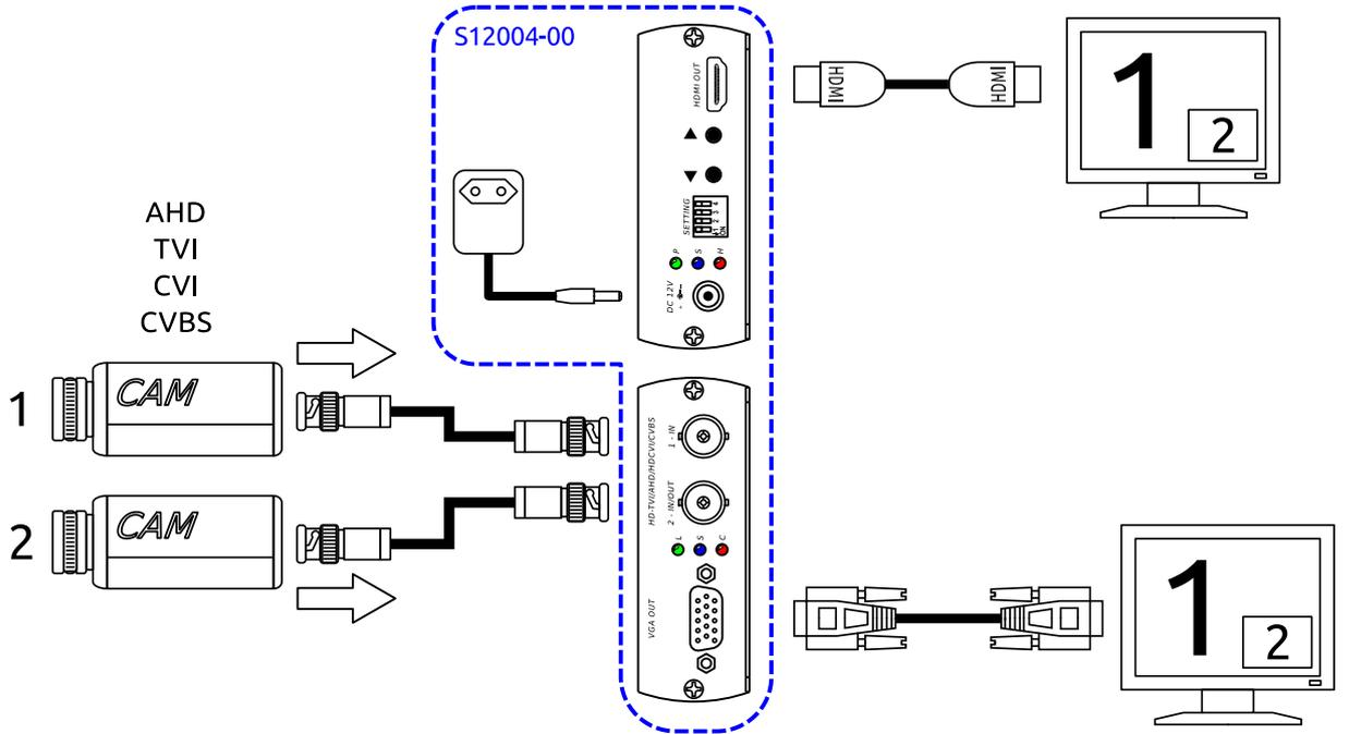
**Câblage 1 BNC en entrée / 1 BNC en sortie**
