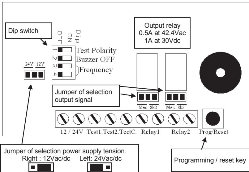
**WARNING:** if the power supply of the TCO7RX is carried out in alternating current (Vac), the power supply must be got through an insulation transformer (of security, SELV tensions) which has a limited power or almost a protection against the short circuit.
